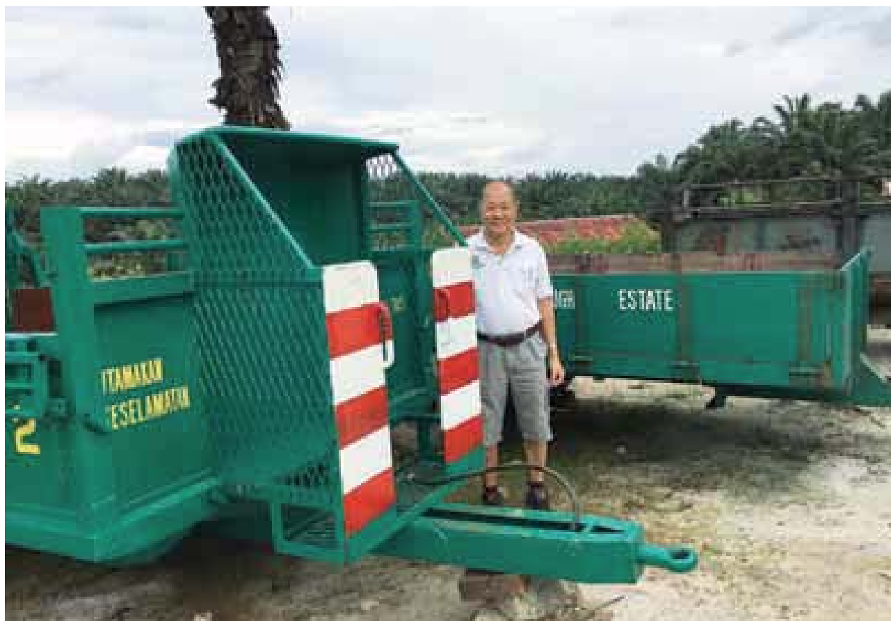
Modified Trailer with Compartment for Harvesters - Narborough Estate
